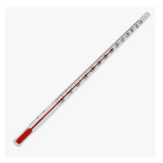
It is a pencil-thin tube of clear glass with graduated temperature readings with a hairline bore through its middle through which the indicator liquid rises.
