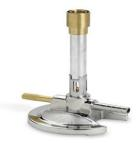
The bursen burner produces a single clean, steady, sootless flame of high temperature, and that's why it is so well-favored in laboratories. It is relatively safe to use when used with caution. Most burners are connected by gas hoses to a single distribution point on a lab workbench, which includes internal plumbing for the gas distribution network.
